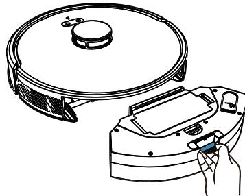
2. Press and hold the dustbin lock to open and dump the dirt inside.
