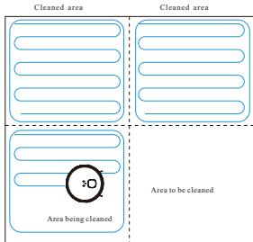
2.Based on the existing area divisions, Robot Vacuum will clean along the edges to form a closed area first and fill in the area in a Z-shaped manner, then clean the remaining areas one after one.
