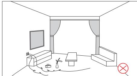
Please sort out the wires, debris and fragile, unstable, valuable and potentially dangerous objects on the ground before starting the device.
