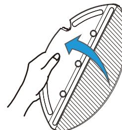
4. Install the holder to the bottom of 2-in-1 dustbin & water tank.
