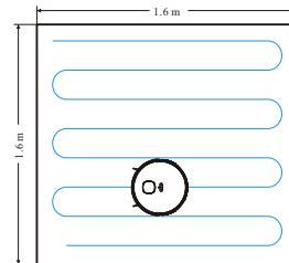
3.Robot Vacuum will move to the designated location and clean an area of  $1.6\text{m} \times 1.6\text{m}$  square with itself as the center twice, then return the charging base for recharging.
