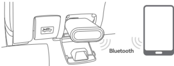
Open the Dollarfix App, and it will automatically search for activated devices. Select your device and connect to it via Bluetooth within the app.
